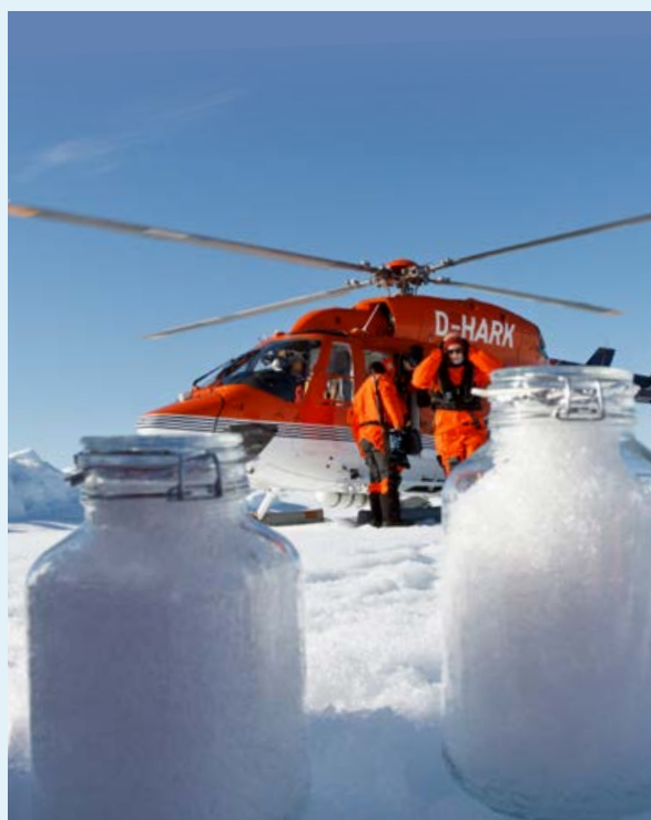
Snow sampling for the assessment of atmospheric microplastic. The sampling took place on a sea ice floe in the Fram Strait during the research expedition PS107 of the German research icebreaker Polarstern (Bergmann et al., 2019). © Kajetan Deja
